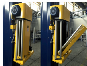
MOTORIZED PRE-STRETCHING AT 200% * (* upon request)
